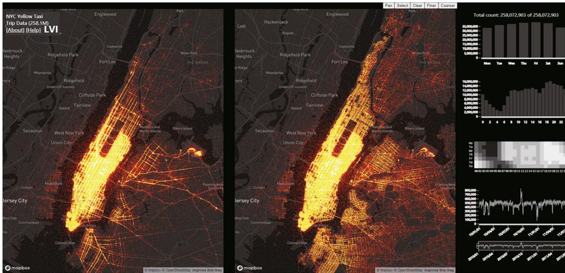
**Fig. 13** A system for analyzing O-D patterns of the taxi-yellow dataset. Longitudes and latitudes of the two maps are uniformly divided into  $2^{25}$  bins to enable high-resolution query/display
